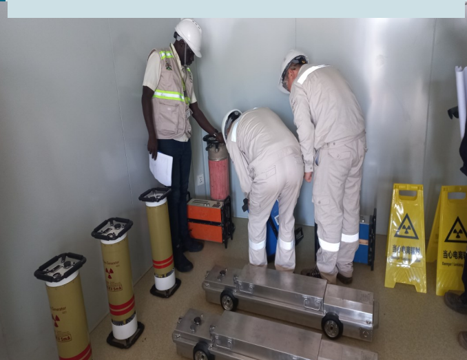
Fig 5: An AEC inspector conducting an Industrial radiography Inspection at a facility.
