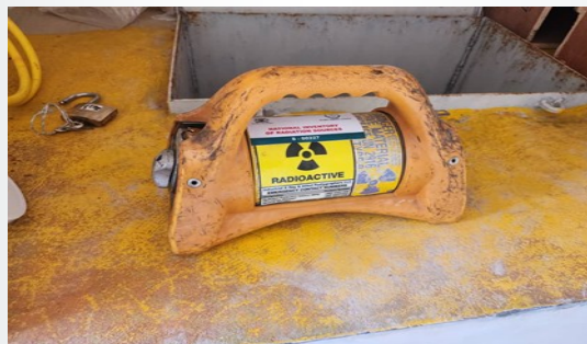
Fig 4: Iridium-192 Gamma Camera Industrial Radiographic Device
