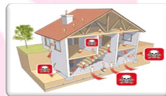
Figure 2: Radon exposure pathways
