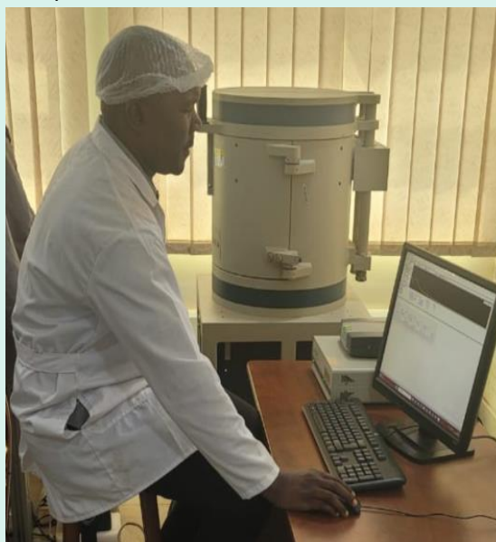
Figure 4: AEC staff analyzing water samples using the High Purity Germanium Detector
